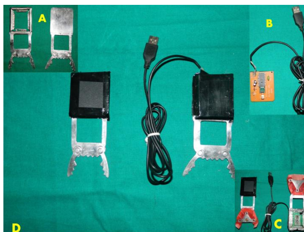
Figure 1:Assembling of the device. Gothic arch tracers with modified maxillary ramp (A) Circuit board of a mouse along with cord (B) Circuit board on the maxillary tracer (C) Sealed mouse modified tracers.
